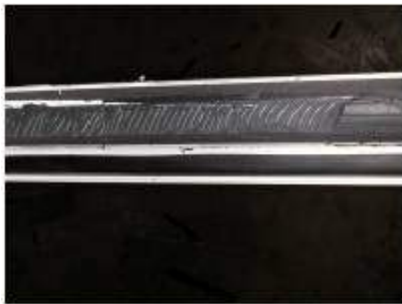
Sealant failed by cohesion in peel adhesion test
